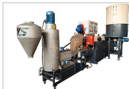
SSFigure 17- Schematic of Single Screw Forced Feeder Type Recycling Extruder (Source https://www.recycleplastics.in )
