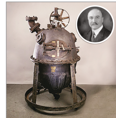
Picture 3- Bakelizer, used by Baekeland (1907- 10) to form Bakelite. Source https://www.sciencehistory.org/historical-profile/leo-hendrik-baekeland
