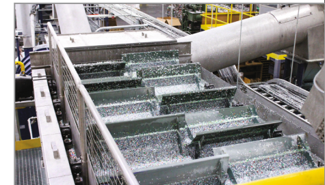
Figure 5 - Sink and Float Separator (Source - B+B Anlagenbau)
