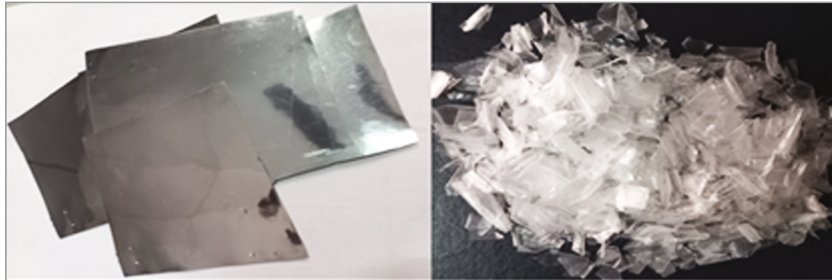
Figure 22 - Demetallizing of films; Before and After (Source: www.recycleplastics.in )
