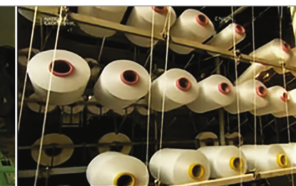
Figure 19- Polyester Fiber being wound on Bobbins (Source: National Geographic)
